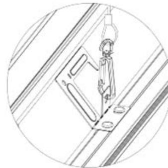
4. Hang the hooks of the suspension ropes into the clips.
